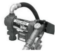
This contractor grade pump with explosion proof UL approved motor pumps Up to 20 GPM. Built using heavy duty cast iron this pump has a 2" threaded base for tank mounting, cast bronze rotor with bronze rotary vanes, and built in strainer. 2 Year warranty.
