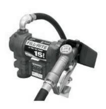
This standard duty 1/4 HP explosion proof UL listed pump can pump Up to 15 GPM. Has a 2" threaded base for tank mounting, cast bronze rotor with bronze rotary vanes, and built in strainer. 2 Year warranty.
