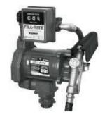
Heavy duty UL listed explosion proof 1/3 HP motor. 807C Meter. Heavy duty switch, thermal overload protection and junction box. Carbon vanes and ceramic/carbon seals. Integral check valve with pressure relief on outlet side. Easy removable strainer, automatic bypass valve, 2" threaded bung for tank openings. 2 Year warranty.
