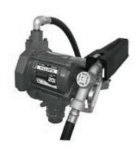
Heavy duty UL listed explosion proof 1/3 HP motor. Heavy duty switch, thermal overload protection and junction box. Carbon vanes and ceramic/carbon seals. Integral check valve with pressure relief on outlet side. Easy removable strainer, automatic bypass valve, 2" threaded bung for tank openings. 2 Year warranty.
