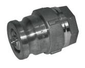
Helps to prevent liquid spillage during the connection/disconnection process. The adaptor contains a spring loaded poppet to assure fast closing and tight seal. Available in 2" or 3" with Buna or Viton Seals.
